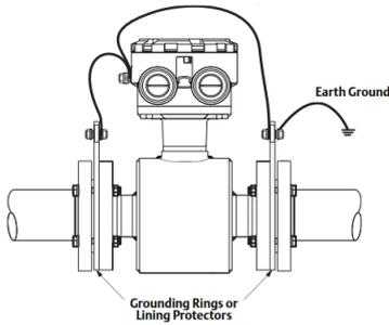
SUITABLE FOR NON CONDUCTIVE PIPE, SUCH AS PVC, USING GROUND RINGS
