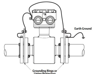
SUITABLE FOR CONDUCTIVE PIPE USING GROUND RINGS
