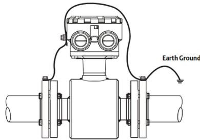
SUITABLE FOR CONDUCTIVE PIPE WITH GROUND ELECTRODE
